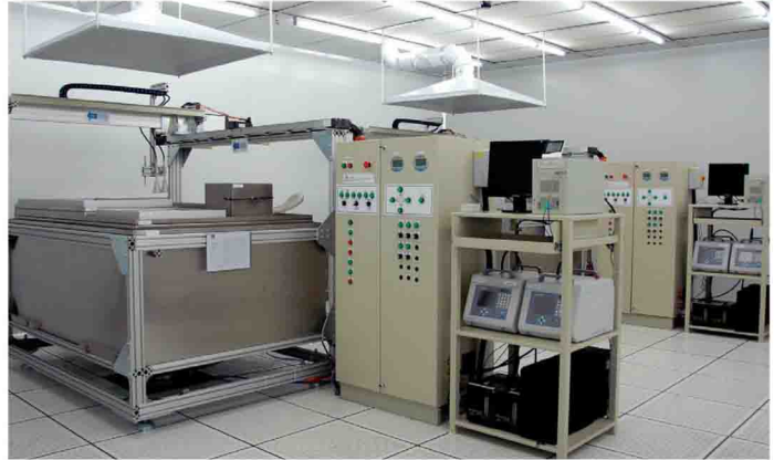
AAF's testing procedures for overall efficiency include laser particle counters with liquid or solid aerosol challenge. Pinhole leaks can be detected using either AAF's proprietary static scan test or automatic scan testing.
